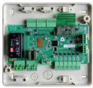
Automation motherboard and Rotenso gateway
